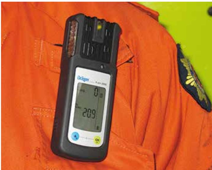
*An important lifesaver for all personnel that have to be inside the plant is to use a personal gas detector that measures both carbon monoxide (CO) and oxygen (O<sub>2</sub>).*
