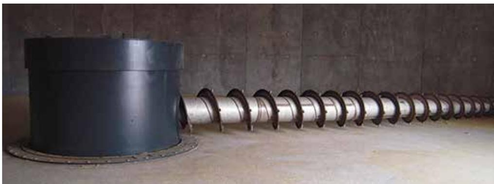
*Examples of free standing concrete and steel silos for biofuel storage/handling. Depending on the type of material used, a rotating screw reclaimer might be used at the bottom of the silo.*
