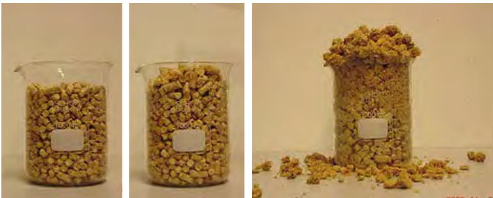
*Wood pellets swell immensely when sprayed with water and may create a very high pressure against the silo wall and result in bridging or hanging. The result is a very hard cake with the same characteristics as a thick particle board that may need to be removed using machinery equipment.*
