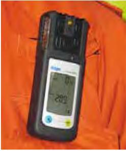
may even be present in personnel areas, control rooms, etc. Measuring instruments that show both carbon monoxide (CO) and oxygen (O<sub>2</sub>) levels should be used to continuously assess the risk area. Measuring instruments must be calibrated regularly. When in doubt, use full protective gear. See more in chapter 3.
