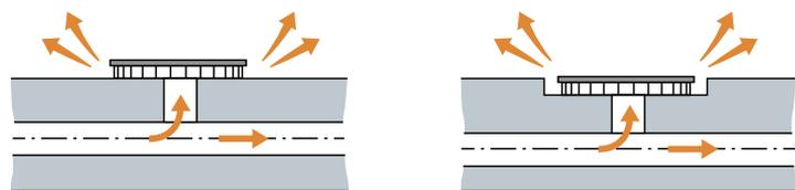
*Gas pipe and gas inlets embedded in the silo floor.*
