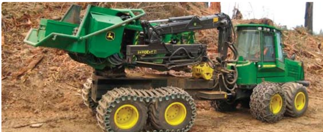
Figure 10: The 'bundler' unit mounted on a forwarder frame can move through the cutover, picking up branch size residue and compressing them into bundles.
