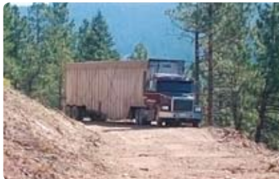
Figure 45: A 'possum-belly' semi-trailer such as this can be used in a set-out system.
