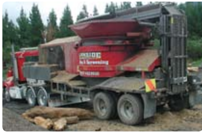
Figure 57: A tub grinder opened up for maintenance on the hammers.
