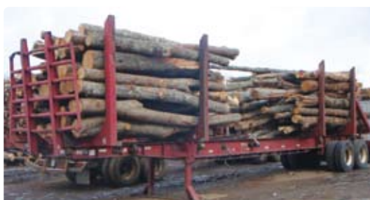
Figure 43: A set-out semi-trailer loaded with logs to be chipped.
