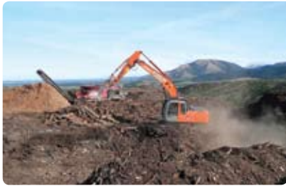
Figure 58: The excavator retrieving and piling the larger residue. The pile was then hogged through the tub grinder.
