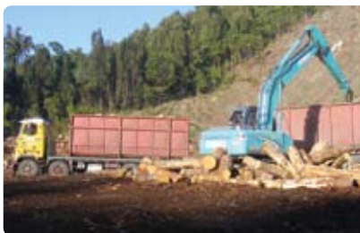
Figure 59: Recovering biomass from the landing and cutover and loading it into a bin truck.
