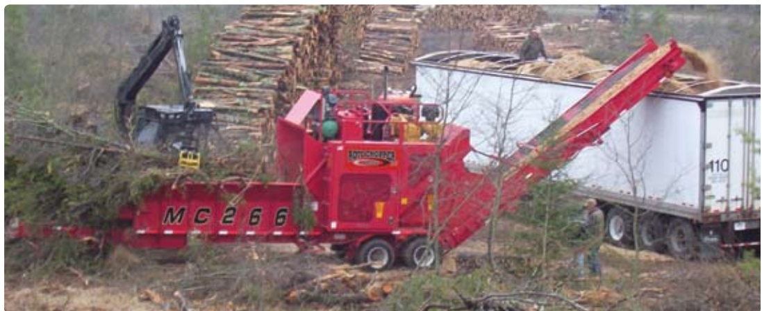
Figure 4: A large scale European wood chipping operation working with a stack of dried logs.
