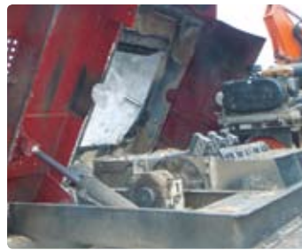
Figure 34: Horizontally-mounted hammers inside a tub grinder.
