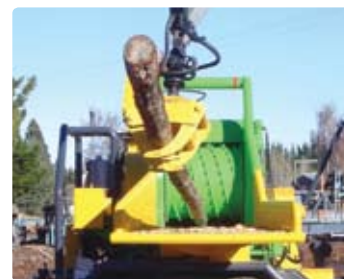
Figure 32: A small but efficient chipper that is powered by the PTO of an agricultural tractor. These systems are relatively cheap to run but limited in the maximum diameter they can cope with.
