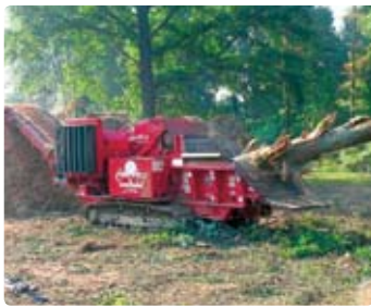
Figure 33: A truck mounted Starchl hogger working with landing slash.
