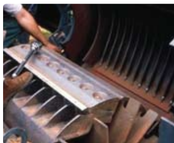
Figure 31: Fixed knives on a drum chipper. The alignment is critical to good operations.
