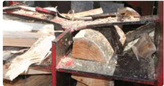
Figure 40: Splitting frame on a firewood machine.
