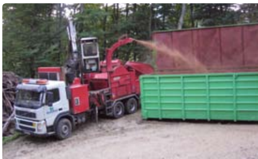
Figure 41: Chipping directly into a set-out bin. This can be effective when cleaning up multiple landings as the trucking and comminution operation is de-coupled.
