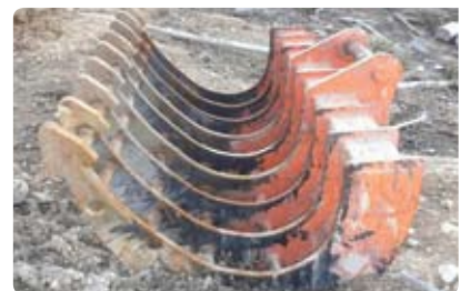
Figure 26: A root-rake that is mounted on an excavator base so the operator can shake out contaminants and under-sized wood residues.
