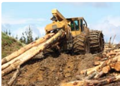
Figure 2: A skidder pulling stems to the landing.
