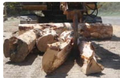
Figure 23: An excavator splitting logs prior to stacking to improve drying.
