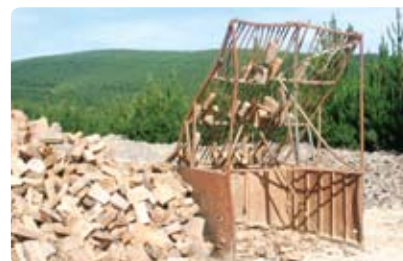
Figure 26: A simple screen used to limit undersize firewood and help remove any dirt contamination.
