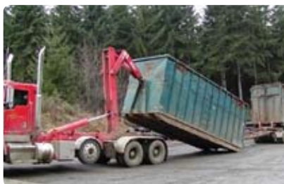
Figure 54: Set-out bins and hook truck and trailer (end loader).
