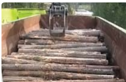
Figure 49: Stacking logs carefully into a bin provides for a loading factor of about 60%. Simply throwing in the wood fuel will only achieve a 30-40% loading factor.
