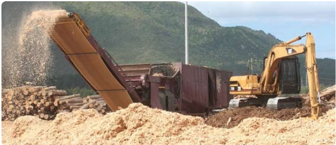
Figure 50: Large scale comminution operations at a CPY where stem residues are being shredded into hog fuel.
