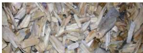
Fig. 16: The dry wood fuel – hogged and screened pallets, with all nails removed.
