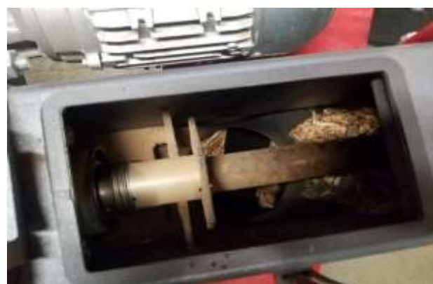
Fig. 29 and 30: The flap to allow ‘strands’ of wood to be removed, and the special design at the top of the auger shaft to knock these strands down
