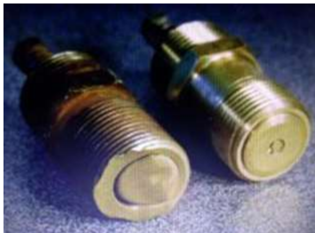
Worn nozzles can also plus as fines material enters the nozzle itself.
