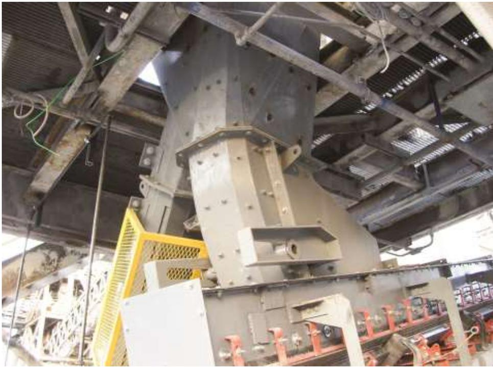
The rear chute wall in this image is bolted onto side flanges, allowing safer access.
